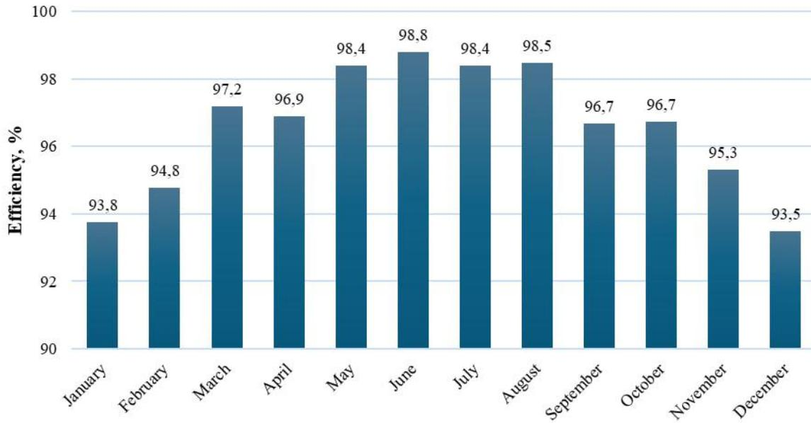
Fig. 3. Results of simulation of the incremental conductance MPPT algorithm for the CdTe/CdS/ITO structure over a one-year period
