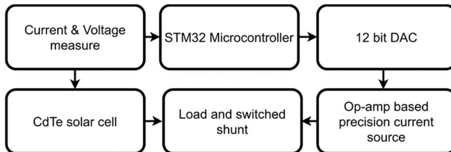
Fig. 2. Block diagram of the MPPT controller
