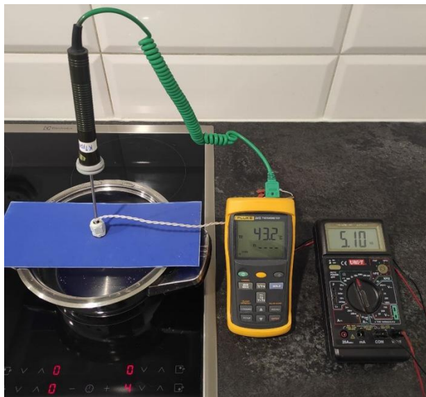
Fig. 4. Calibration of thermistors in a water bath.
