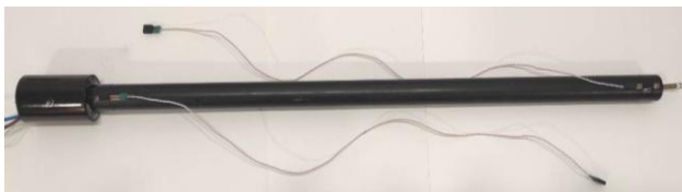
Fig. 5. External view of a heat pipe with a power amplifier and temperature sensors.
