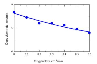
**Fig. 2.** ITO50 film deposition rate at different  $Q(O_2)$ .
