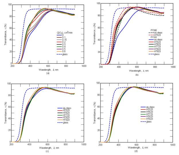
**Fig. 4.** Effects of  $Q(O_2)$  on the transmittance of as-depo. ITO50 (*a*) and  $T_{HT}$  on the transmittance of ITO50 deposited in pure Ar and comparison with  $\tau$  curves of as-depo. and HT523 ITO90 obtained at  $Q(O_2)=0.2 \text{ cm}^3/\text{min}$  (*b*) and  $T_{HT}$  on the transmittance of ITO50 deposited at  $Q(O_2)=0.3 \text{ cm}^3/\text{min}$  (*c*) and  $T_{HT}$  on the transmittance of ITO50 deposited at  $Q(O_2)=0.4 \text{ cm}^3/\text{min}$  (*d*).
