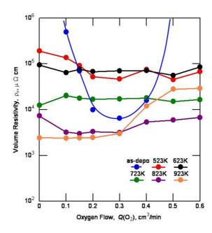
Fig. 3. Effects of  $Q(O_2)$  and  $T_{HT}$  on the volume resistivity of ITO50 thin films.
