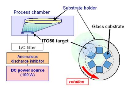
Fig. 1. Schematic diagram of the sputtering apparatus.
