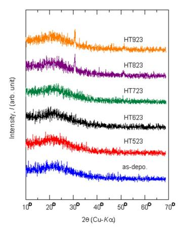
Fig. 5. XRD results for ITO50 films deposited at  $Q(Ar)/Q(O_2) = 50/0.3 \text{ cm}^3/\text{min}$ .
