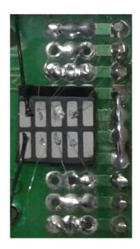
**Fig. 4.** Ag/Ag<sub>8</sub>SnSe<sub>6</sub>/C resistive switching cell.
