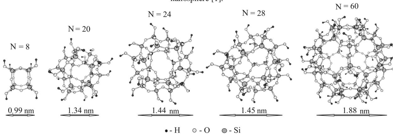
**Fig. 2.** Equilibrium spatial structure of the hollow spherical silica molecule  $(\text{SiO}_2)_N(\text{H}_2\text{O})_{N/2}(\text{SiO}_2)_N(\text{H}_2\text{O})_{N/2}$ .
