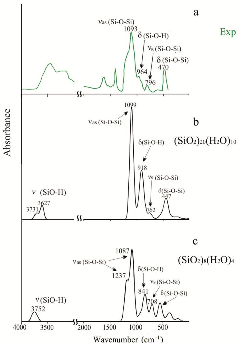
**Fig. 3.** Experimental (a) IR spectrum of the hollow nanospheres of silicon dioxide [8]; the calculated (b) IR spectrum of the molecule  $(\text{SiO}_2)_{20}(\text{H}_2\text{O})_{10}$  and the calculated (c) IR spectrum of the molecule  $(\text{SiO}_2)_8(\text{H}_2\text{O})_4$ .
