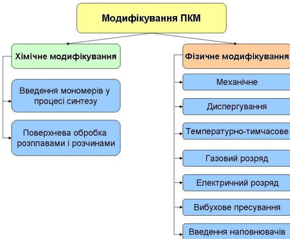
Fig. 1. Scheme of the main methods of modification PCM based on PTFE.
