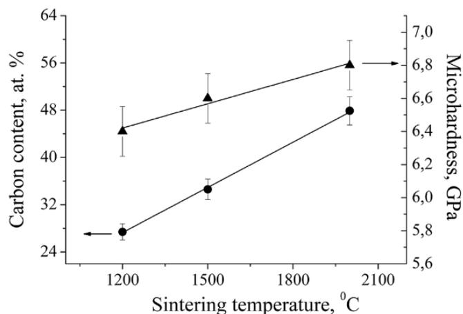
**Fig. 3.** Microhardness of HT-HP sintered Ni-CNT (3:1) samples and a carbon content in a charge.
