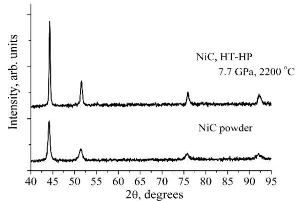
**Fig. 1.** Diffractograms of mechanically alloyed Ni-Graphite (1:1) charge and a sample sintered from it.
