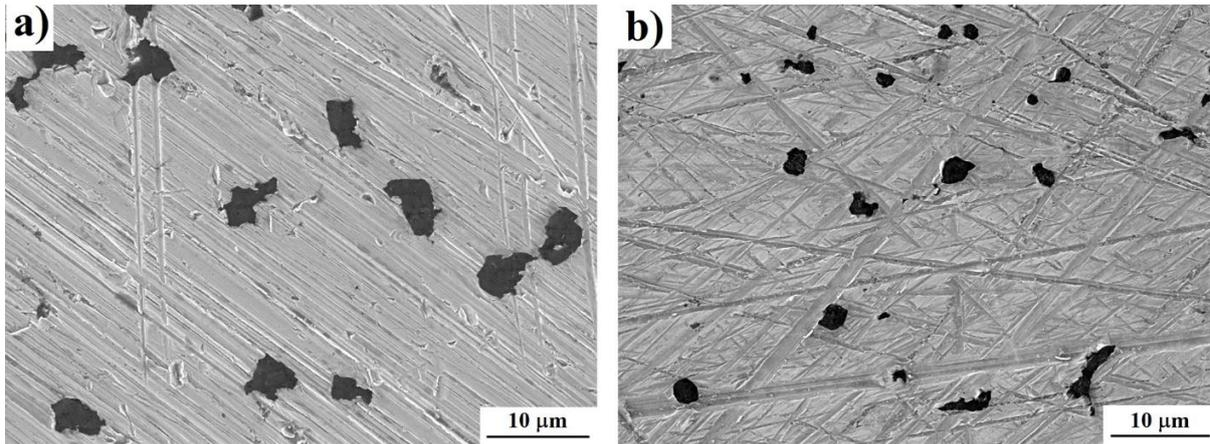
**Fig. 2.** SEM images of HT-HP sintered (7.7 GPa and 1850 °C) samples: (a) Ni-graphite (1:1); (b) Ni-CNT (1:1). x2000.
