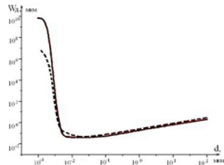
**Fig. 4.** Domain width  $W_d$  dependencies from the thickness of the epitaxial film: (simulation results) [18].
