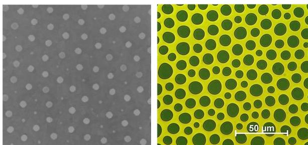
**Fig. 5.** The image of the cylindrical domain structure of the YIG.
