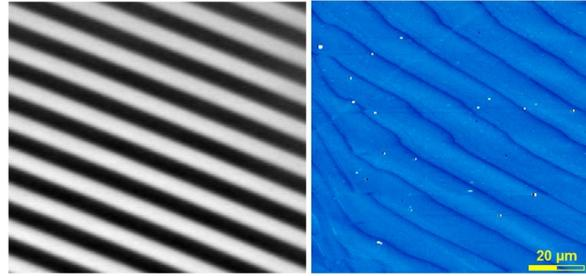
**Fig. 3.** Image of the strip domain structure of the YIG films.
