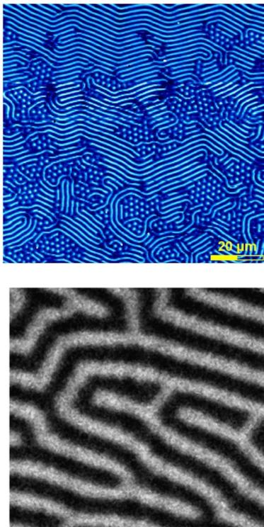
**Fig. 2.** Image of the labyrinth domain structure of the YIG films.
