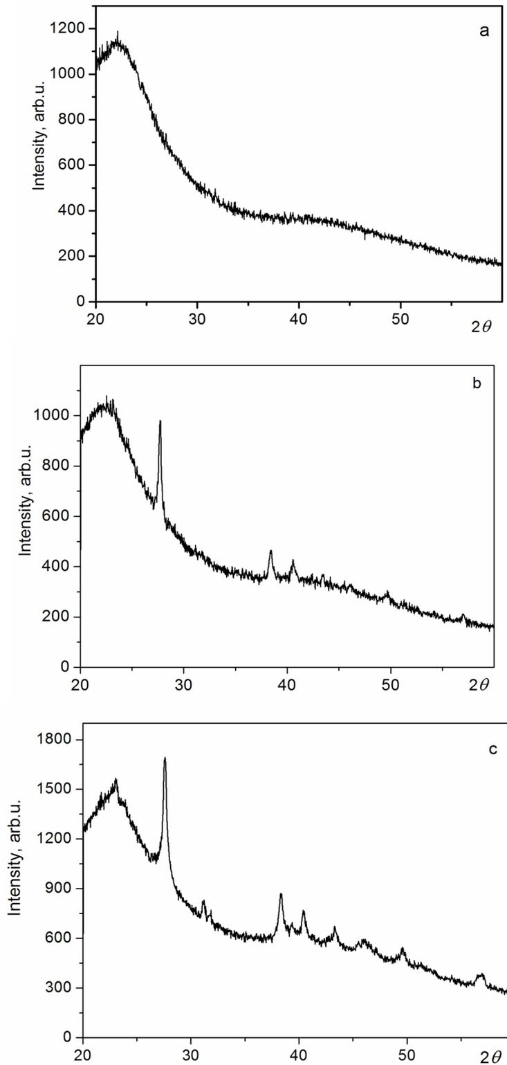
**Fig.2.** X-ray diffraction images of dispersed samples of K:Cd A:Te(a), K:Te A:Cd(b), K,A:CdTe(c) systems.
