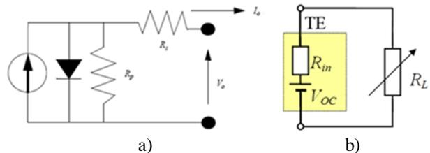
Fig. 4. Equivalent electrical circuit of the photoelectric cell (a) and thermoelectric module (b).
