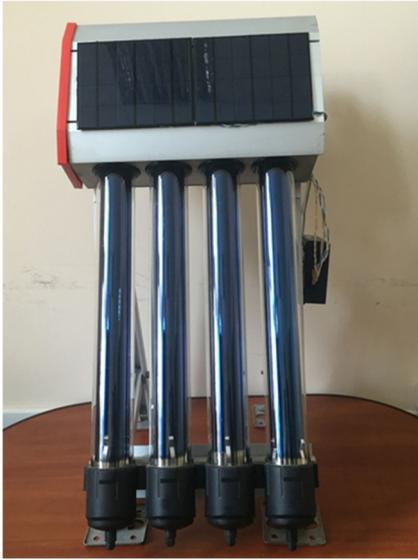
**Fig. 1.** Photograph solar thermoelectric generator.
