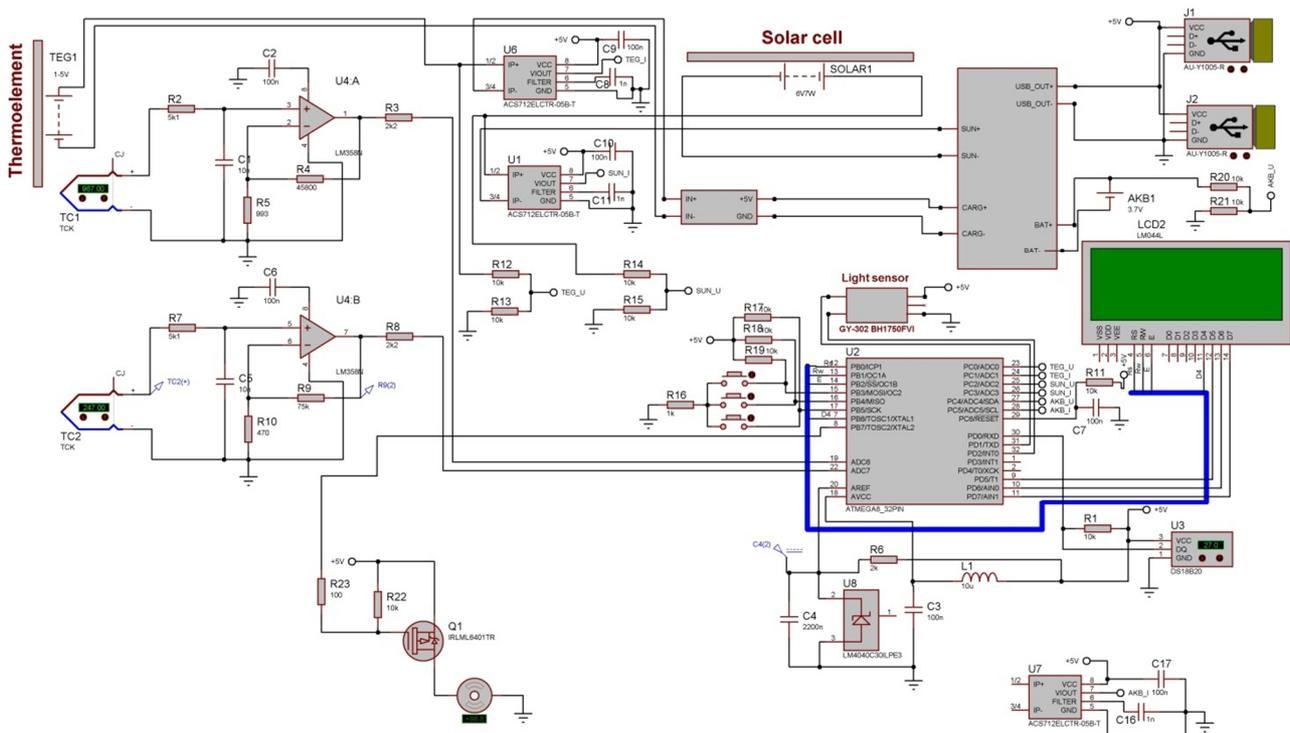
Fig. 3. Electric diagram of the control system.
