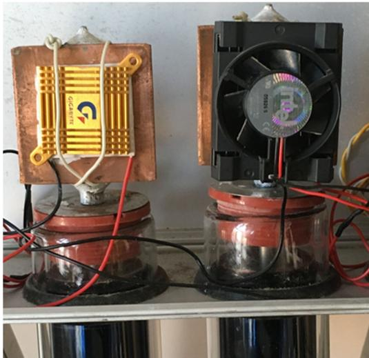
**Fig. 2.** Photo with thermoelectric module occur on the condenser of vacuum collector.
