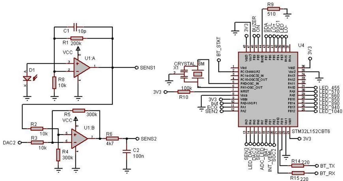
**Fig. 2.** Functional principle scheme of the signal converter from photosensitive elements for photoplethysmography.
