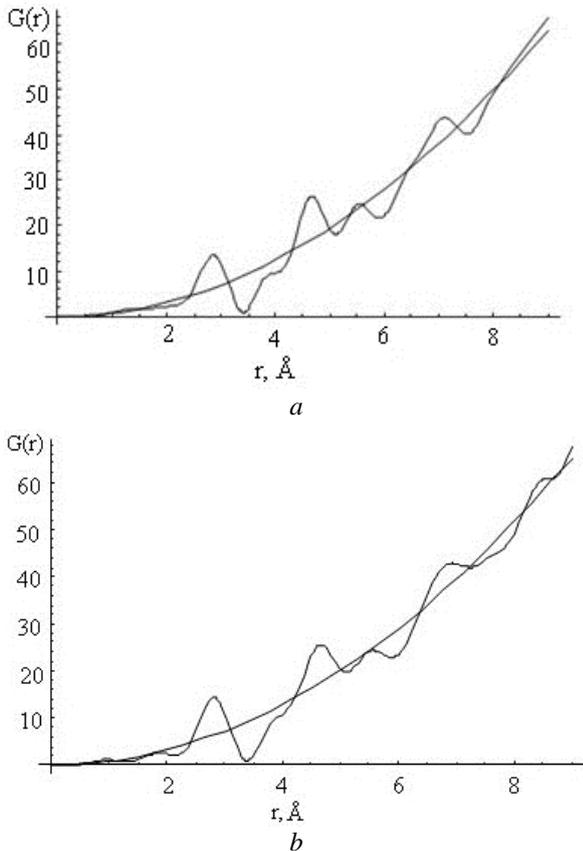
**Fig. 2.** RDF of atoms for alloys: (a)  $Co_{84}W_{16}$ ; (b)  $Co_{88}W_{12}$ .
