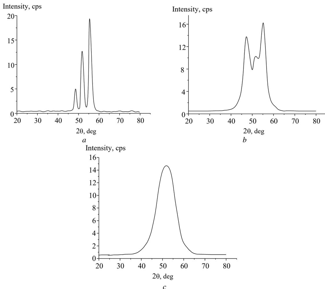
Fig. 1. Intensity of scattering by substances: (a) Co; (b) Co<sub>90</sub>W<sub>10</sub>; (c) Co<sub>84</sub>W<sub>16</sub>.
