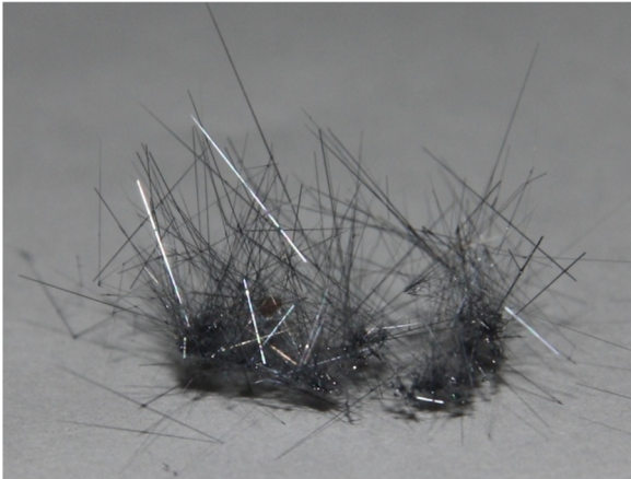
Fig. 2. Type of a bundle of \text{Si}_{0.97}\text{Ge}_{0.03} whiskers.
