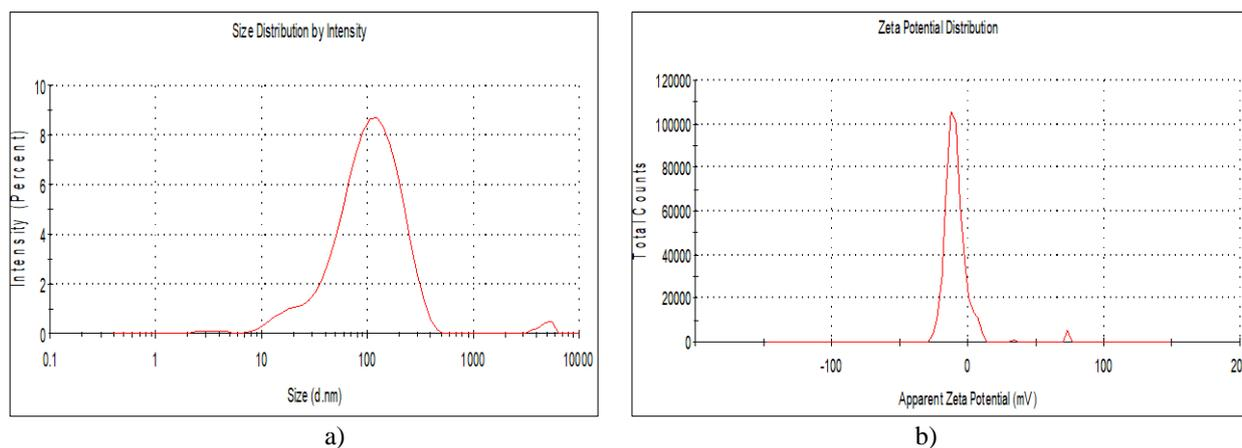
**Fig. 3.** DLS image (a) Size distribution (b) Zeta potential of bioengineered Ag NPs.
