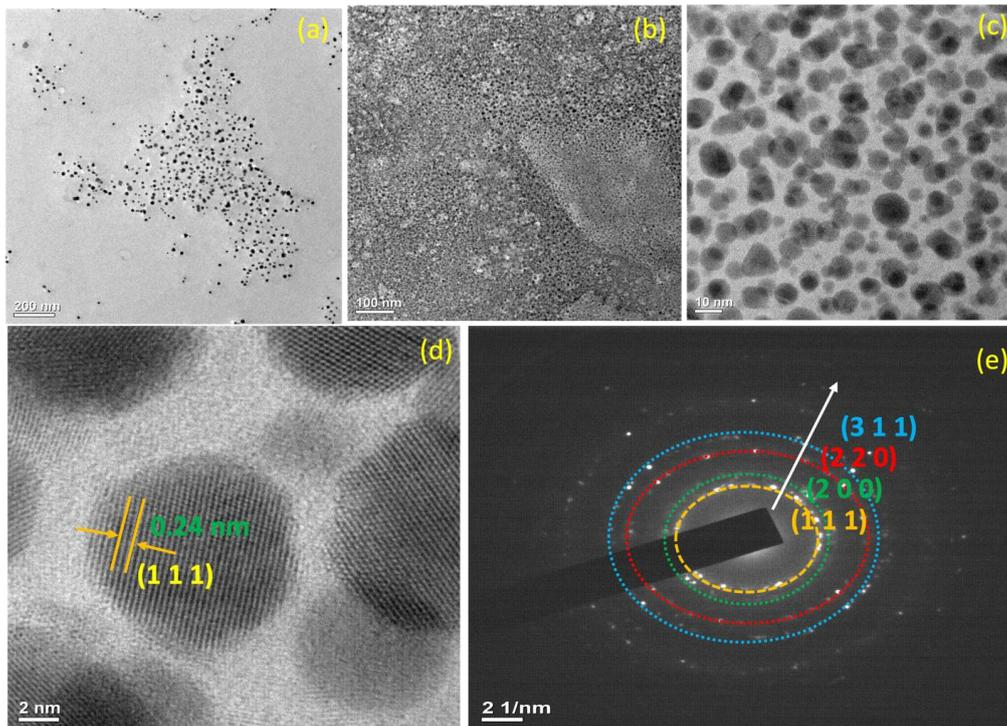
**Fig. 5 (a-c).** TEM Images with different magnifications (d) d-spacing image, (e) SAED pattern of the prepared bioengineered Ag NPs.
