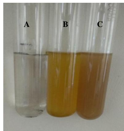
**Fig. 1.** Change in the colour of the colloidal solution after incubation with 5mM  $\text{AgNO}_3$  solution A –  $\text{AgNO}_3$  solution, B – Plant extract, C – Silver nanoparticles solution.
