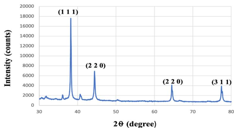
**Fig. 7.** XRD pattern of bioengineered Ag NPs.
