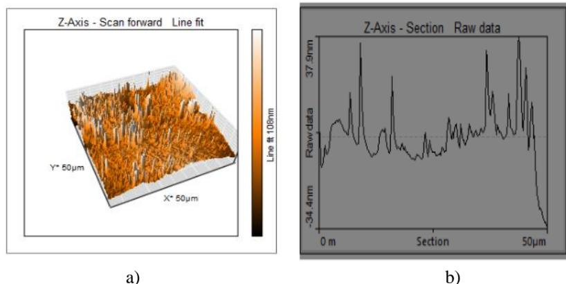
**Fig. 2.** AFM image (a) Topography and (b) Deflection pattern of bioengineered Ag NPs.
