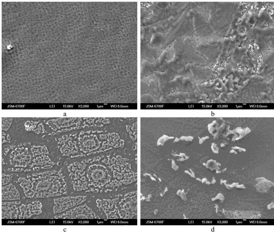
**Fig. 2.** SEM image of the titanium nanofilms on the ZrO<sub>2</sub>-ceramic after annealing in vacuum at 1500°C with different holding time: a – 2 min; b – 5 min; c – 10 min; d – 20 min.
