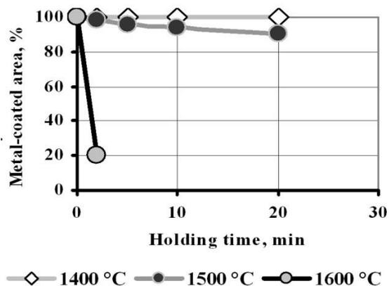
**Fig. 12.** Kinetics of the hafnium thin films coagulation on zirconia.
