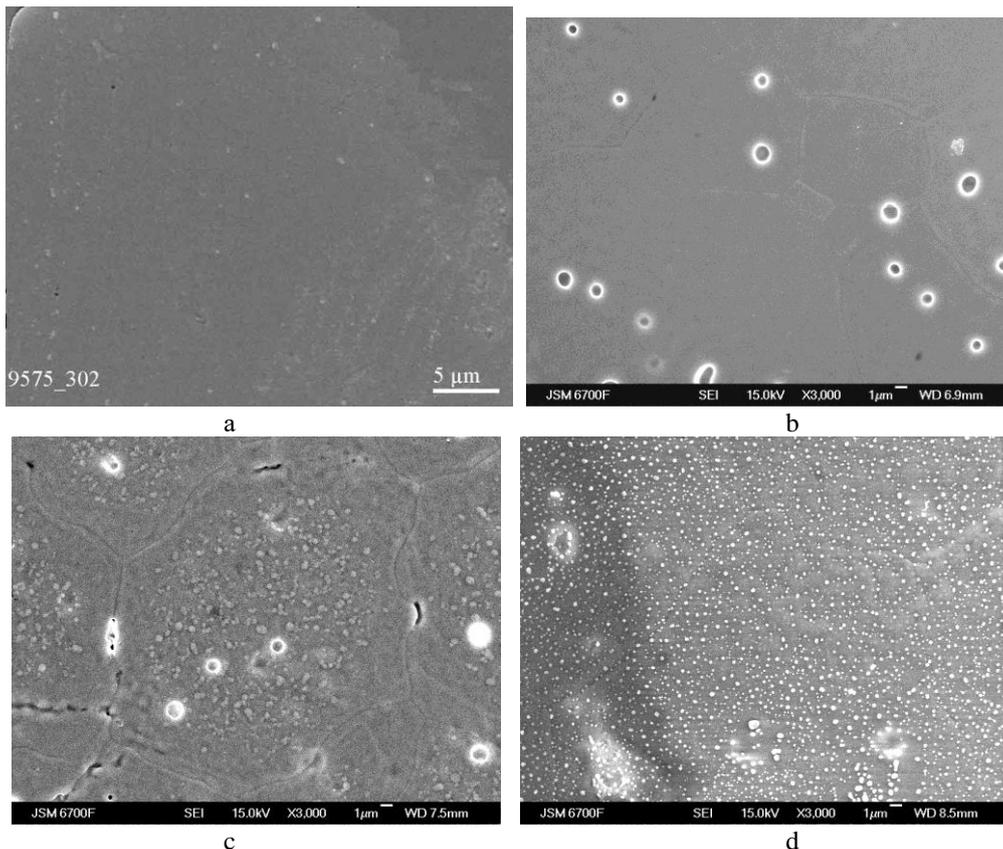
**Fig. 9.** SEM images of the hafnium nanofilms onto the  $ZrO_2$ -ceramic after annealing in vacuum at 1400°C with different holding time: a – 2 min; b – 5 min; c – 10 min; d – 20 min.
