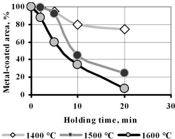
**Fig. 4.** Kinetics of the titanium nanofilms onto zirconia coagulation.
