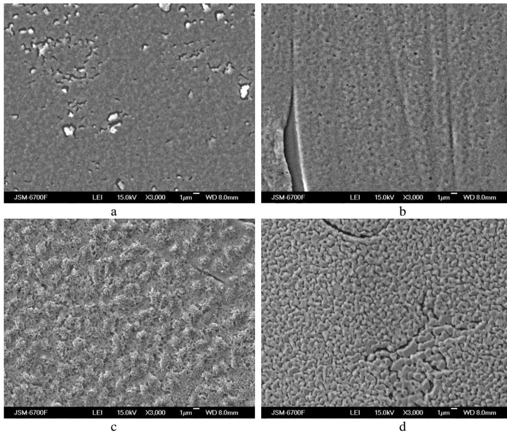
**Fig. 6.** SEM images of the zirconium nanofilms onto ZrO<sub>2</sub>-ceramic after annealing in vacuum at 1500°C with different holding time: a – 2 min; b – 5 min; c – 10 min; d – 20 min.
