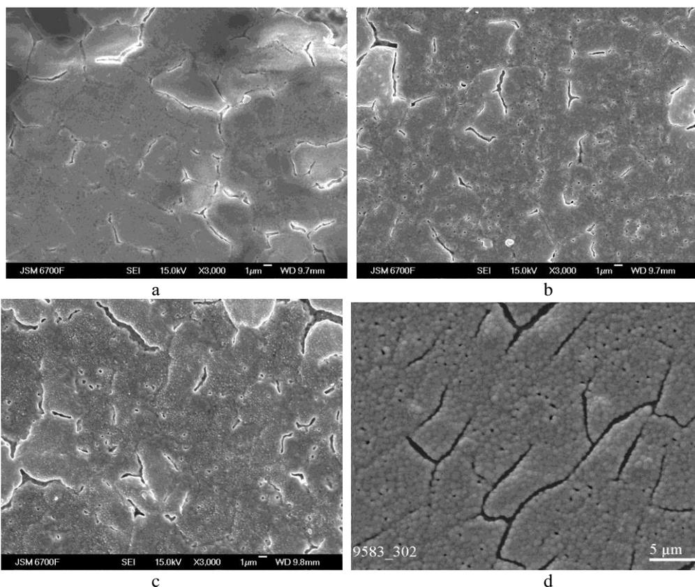
**Fig. 10.** SEM image of the hafnium nanofilms onto the  $ZrO_2$ -ceramic after annealing in vacuum at  $1500^\circ C$  with different holding time: a – 2 min; b – 5 min; c – 10 min; d – 20 min.
