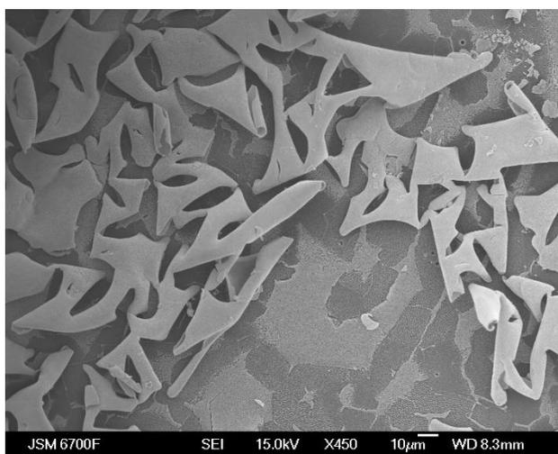
**Fig. 11.** SEM image of the hafnium nanofilm onto the  $ZrO_2$ -ceramic after holding during 2 min at  $1600^\circ C$  in vacuum.
