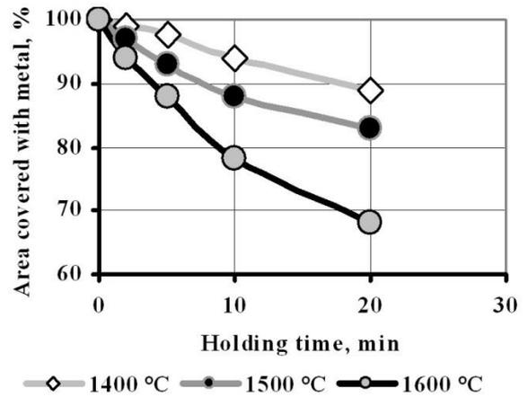
**Fig. 8.** Kinetics of the zirconium nanofilms onto zirconia coagulation.
