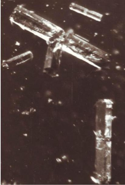
**Fig. 1.** Photograph of gallium nitride crystals taken at  $\times 20$  magnification.
