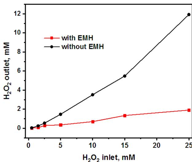
Fig. 3. The relationship between the residual concentration of H<sub>2</sub>O<sub>2</sub> and its initial concentration at the inlet of the ferrite reactor, along with the impact of electromagnetic heating.
