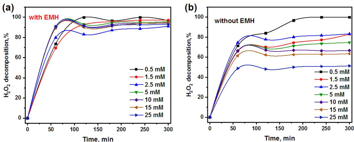
Fig. 2. Efficiency of H<sub>2</sub>O<sub>2</sub> decomposition: (a) with EMH; (b) without EMH.
