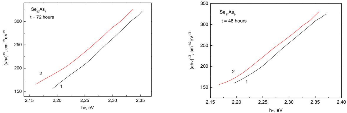
**Fig. 4.** Dependences of the absorption edge  $[\alpha(h\nu) \cdot h\nu]^{1/2}$  on the energy of photons of nominally pure (1) and mercury-modified (2) during  $t = 72$  and  $48$  h of  $\text{Se}_{93}\text{As}_7$  (a) and  $\text{Se}_{91}\text{As}_9$  (b) films.
