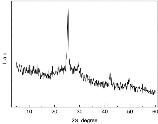
**Fig. 2.** X-ray diffractogram of the mercury-modified for 72 hours amorphous  $Se_{95}As_5$  film.
