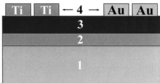
**Fig. 1.** Schematic representation of the structure under study: 1 – silicon substrate, 2 – lower metallization layer, 3 – polymer layer with C<sub>60</sub>, 4 – upper ohmic contacts.
