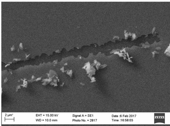
**Fig. 4.** Specifics of the structure of the crystalline ScGe<sub>2</sub> thin film after long aging (X3000).
