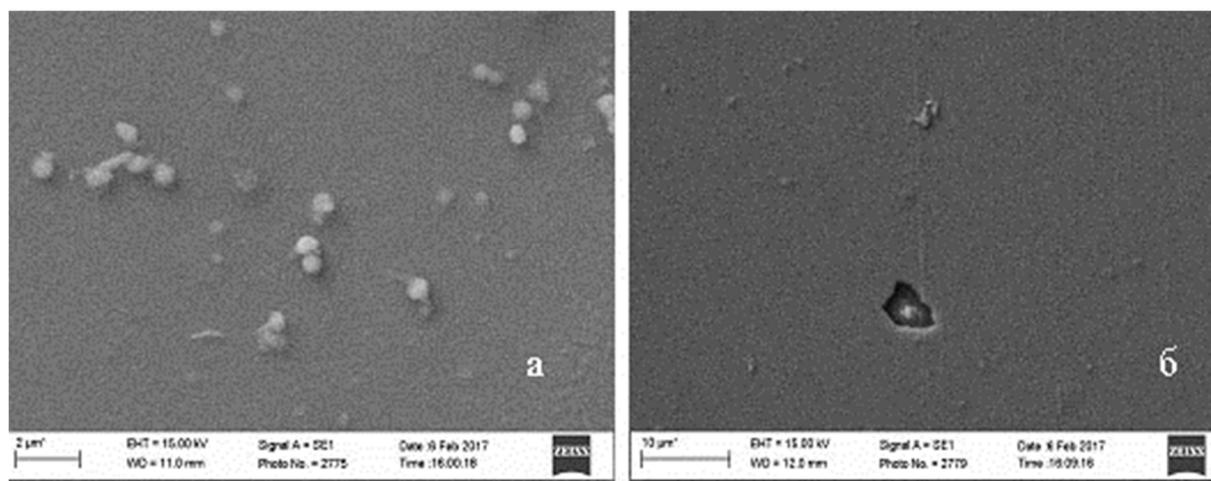
**Fig. 1.** Morphology of  $Y_{25}Fe_{25}Ge_{50}$  thin films, obtained by  $v_p = 6$  nm/sec and  $T_p = 710$  K by coevaporation, after long aging in desiccator (a - X6000; b - X2000; the scale in the left corner micrographs is shown).
