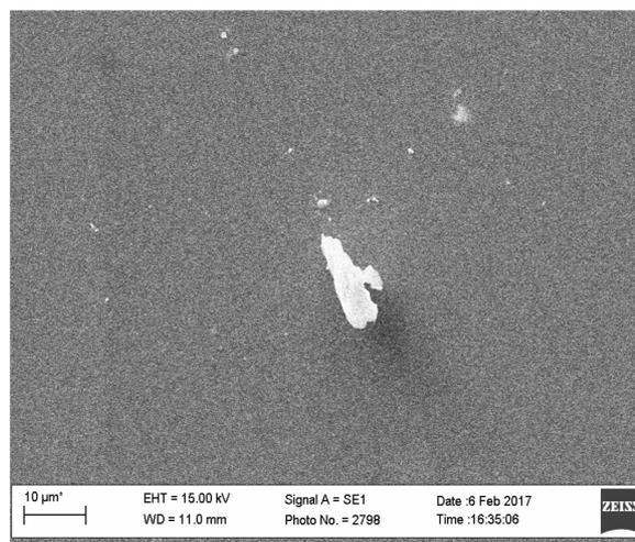
**Fig. 2.** Electron micrograph of crystalline  $LaNiGe_2$  thin films, obtained by discrete evaporation at  $v_p = 5$  nm/sec and  $T_p = 700$  K, after 20 years of aging (X1000).
