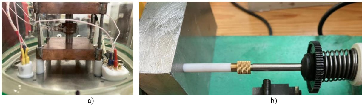
Fig. 1. General view of the measuring cell and configuration of samples for measurement.
