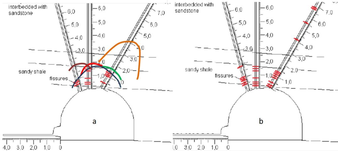
**Fig. 5.** Sequential kinematics of fracture development according to Lubosik et al., 2015: (a), (b) – at the distance 220 m and 12 m in front of the longwall respectively.
