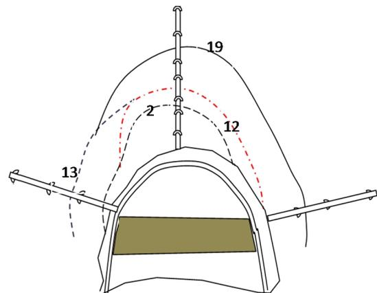
**Fig. 4.** Development of disintegrated zone around underground roadway.
