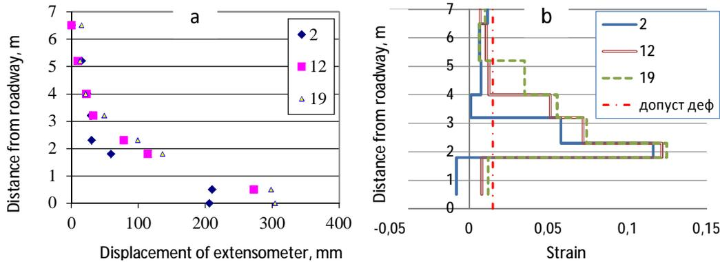
**Fig. 3.** Subsidence of the roof (a) and extension of intervals (b).
